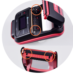
Black Mark and Gap Detection
